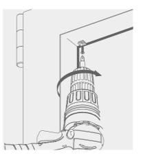
Fit the blind using cord fasteners.
