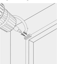
Attach the brackets onto the fasteners.
