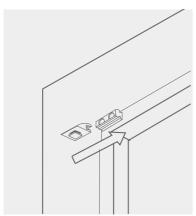
Fit the blind using cord fasteners. .
