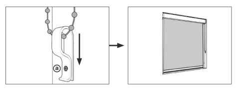
• Secure P clip to the wall recess using screw (a).
